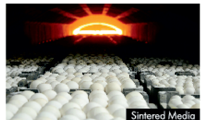
Micro processor controlled high temp. 1650°C gas fired tunnel Kiln
